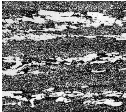
Fig1. Conventional W.Nr. 1.2379 (AISI D2) with Typical lines of primary carbides
